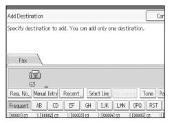
When the file has some Internet Fax destinations, you can switch the transmission type between fax/IP-Fax and Internet Fax by pressing **[Fax]** or **[Internet Fax]**. To add an e-mail address, switch the type of transmission to Internet Fax by pressing **[Internet Fax]**. Then, press **[Manual Entry]** and enter the e-mail address. You can also program a SUB Code or SEP Code by pressing **[Adv.Features]**.
